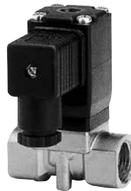
GEMÜ 8257 Servo assisted solenoid valve with a positive lift diaphragm without pressure differential Brass or stainless steel DN 8 - 12 (0 - 10 bar)
